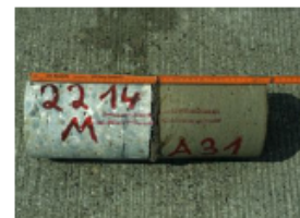
Figure 2. Core from Germany showing nonwoven geotextile interlayer between surface concrete (left) and cement-treated base (right)
